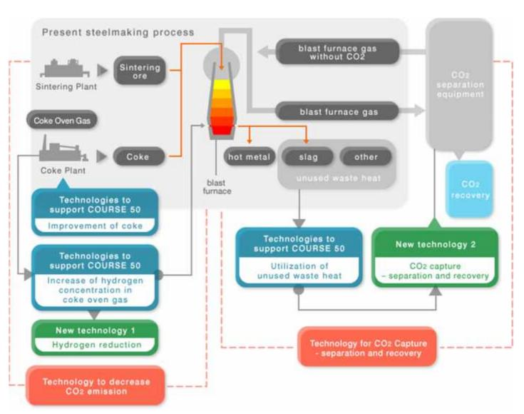
2 CO<sub>2</sub> capture methods are tested:
