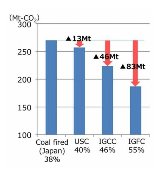
CO<sub>2</sub> reduction potential for coal-fired power plants in the efficiency improvement
